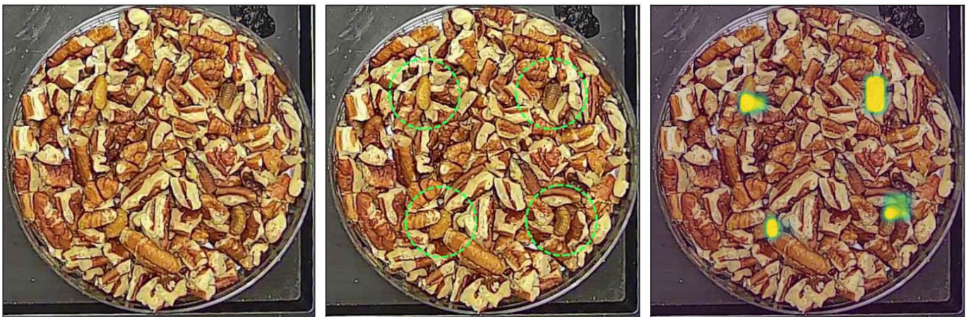
Figure 4: (left) Test dish containing pecan nutmeat pieces and four individual larvae; (center) Test dish with positions of larvae manually outlined by rings with dotted lines; (right) Heat-map result of the machine learning model on the test dish, where 'hot' bright yellow is high probability of larvae
