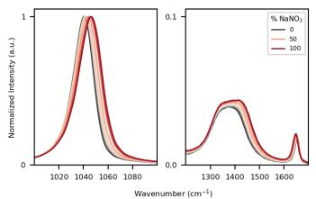
Figure 2: Raman spectra in a range of NaNO<sub>3</sub>/KNO<sub>3</sub> concentrations at 400°C.
