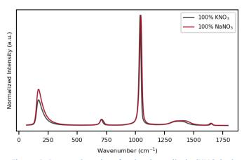
Figure 1: Raman Spectra of potassium nitrate (KNO<sub>3</sub>) at 400°C and sodium nitrate (NaNO<sub>3</sub>) at 400°C
