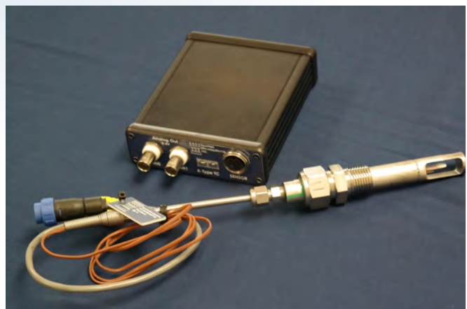
Figure 1. Sporian flow sensor with drive electronics.
